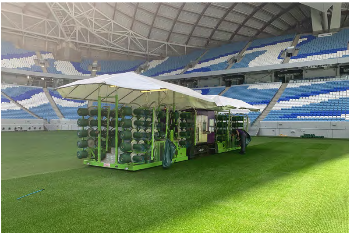
Figure 7: Stitcher used to install stitched hybrid reinforcement systems
